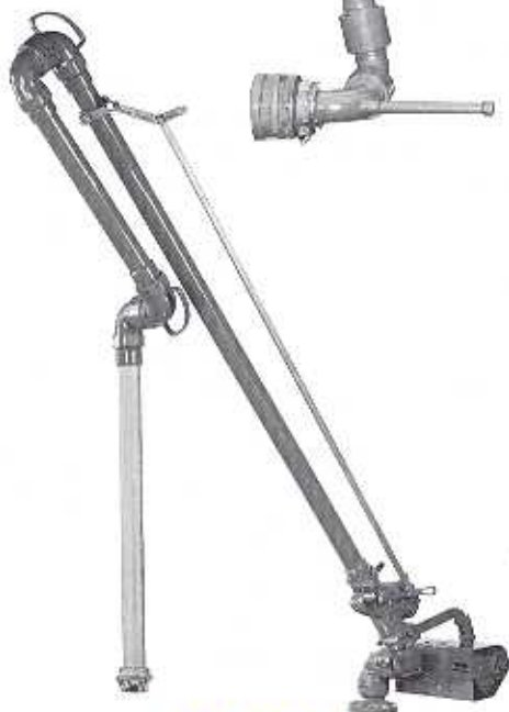
Model E1156 Economical, medium range, dry line, pantograph style, top loader.
